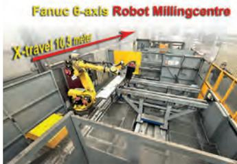
**Fanuc 6-axis Robot Millingcentre**
